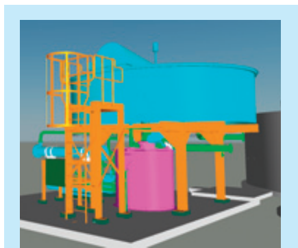
AutoCAD Plant 3D enabled Poole Projects engineers to model the new equipment providing best access for installation and maintenance
