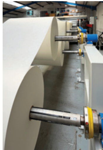
Svecom safety chucks, shafts and Renova pneumatic brakes have been installed at Linwood Raker, UK to provide improved efficiency
