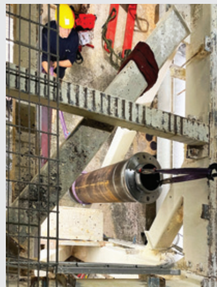
Yankee dryer insulation sleeve inspection and timely replacement by Walmsleys engineers can help protect this high-value asset and preserve machine uptime
