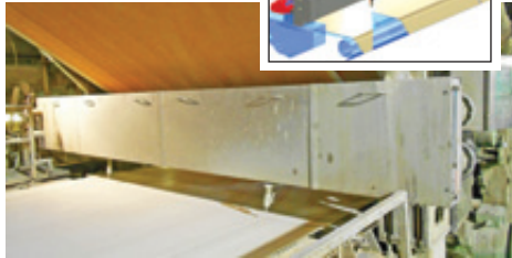
Weingrill tail cutter (TCU-2) with double nozzle ▶
