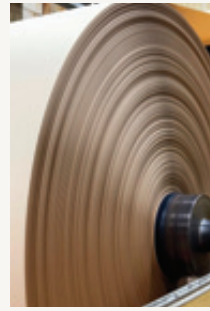
Installation of Compact's Corona dryers has corrected the profile giving nice sharp edges ▶
